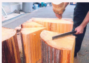
❷ Hand-split multiple times to get thin boards
