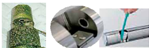
Cleaner with built-in wiper. Maintenance is simple due to the sapphire glass used for the display window.
