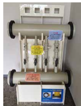
A sample of the designing and welding of a membrane module for low-pressure filtration
