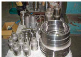
Various components coated by thermal spray technology
