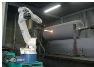
A robot is thermal-spraying the cemented carbide on the surfaces of rolls.
