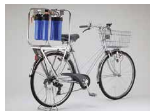
"Mobile Oasis," a bicycle with a water purification system
