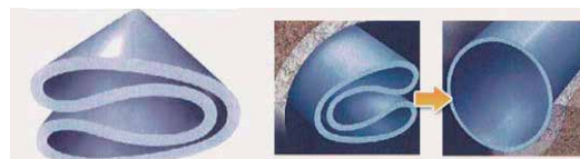
A PVC pipe that memorizes and stores its shape
