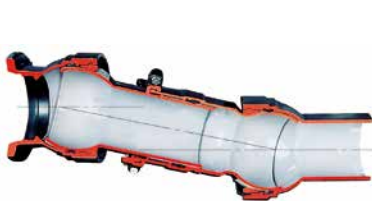
Structure of SUPER FLEX With a dual-structure pipe set between two balls, SUPER FLEX absorbs compound displacement such as deflection, expansion, contraction and torsion.
