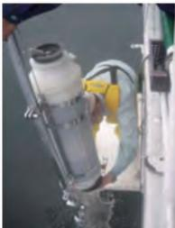
Fig. 4-6-4 Van Don Water Sampler for sampling water at various depths
